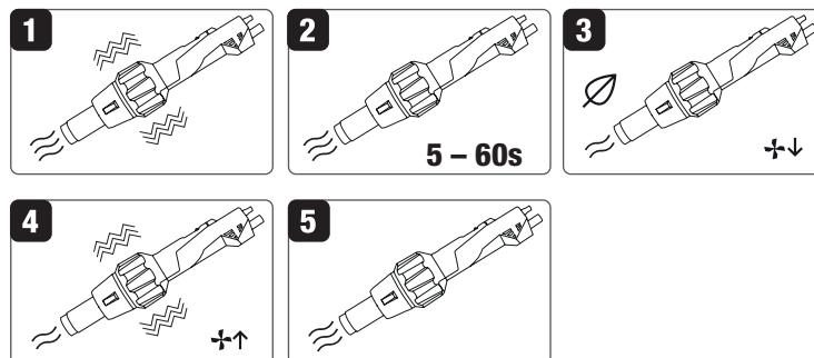
(C5 = 2) Eco 90° tilt angle function turned on (immediat Eco activation if tilt angle = 90°)
